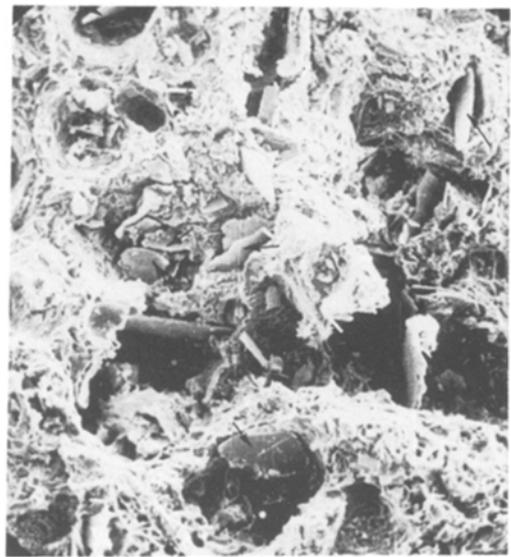
Figure 4 Scanning electron microphotograph of the fractured surface of cut mica dispersed Al-4.0 wt % Cu-1.5 wt % Mg-1.7 wt % mica composite (arrows indicate mica particles) ( $\times 80$ ).
