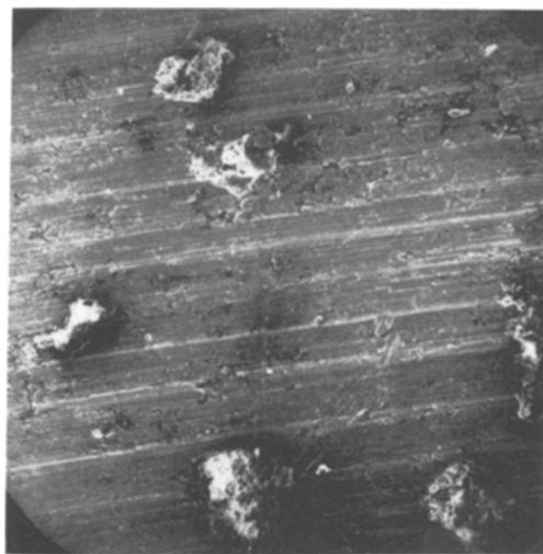
Figure 8 Scanning electron microphotograph of a typical machined surface of Al–4 wt % Cu–1.5 wt % Mg–2.0 wt % mica composite (X 72).
