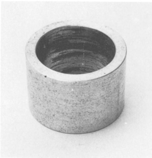
Figure 2 Macro photograph of a typical bearing casting of Al-4.0 wt % Cu-1.5 wt % Mg 1.5 wt % mica composite.
